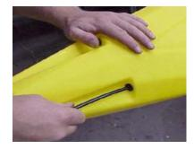
1. Use a knife to cut the ends of the tubing at an angle to make inserting the tubing easier. Lubricate one length of tubing with soapy water and insert it into a stern grommet (5). Push the tubing inside the kayak, leaving a few inches outside.
